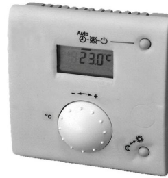
Room unit QAA50.110/101 , with LCD display, room temperature measurement and display, knob for manual setpoint readjustments, operating- and presence button
